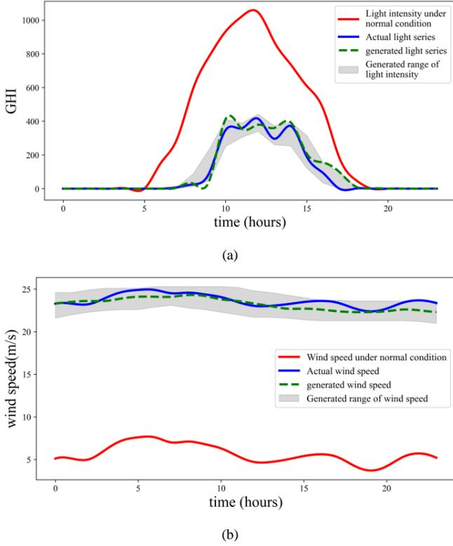
Fig. 4. Solar irradiance and wind speed curves generated by FastGAN
