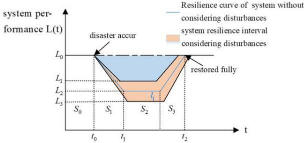
Fig. 2. Schematic diagram of system resilience curve
