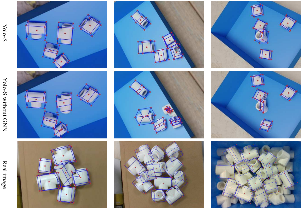
Fig. 3: Texture-less pipe estimation result based on BlenderProc rendered image.
