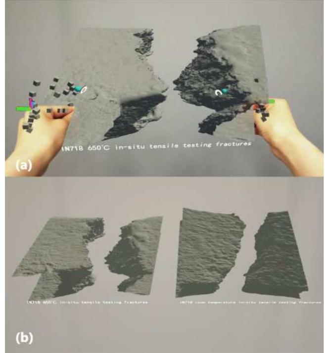
Fig. 7. Interaction and observation of 3D fracture morphology models
