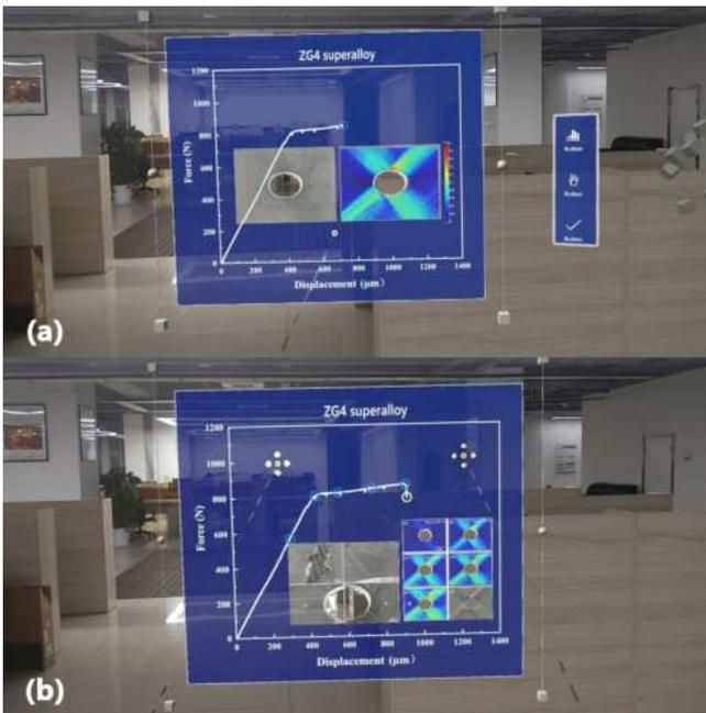
Fig. 6. SEM images and DIC strain distribution images of the film cooling hole at the intermediate and final fracture states
