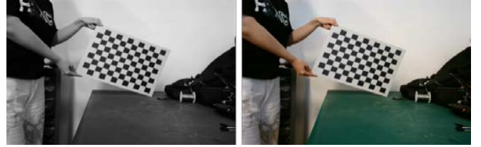
Fig. 8. Near-infrared camera images (on the left) and visible light camera (on the right)
