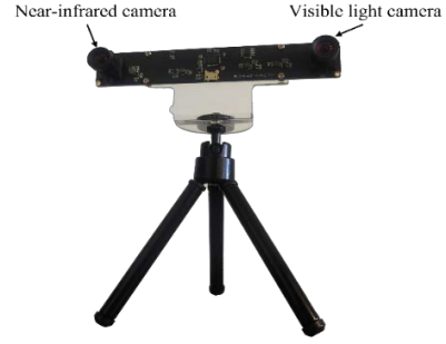
Fig. 7. Visible light and near-infrared binocular camera platform
