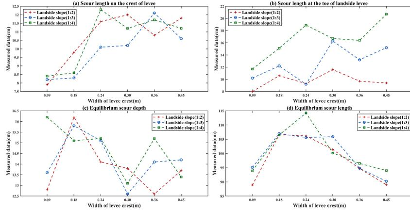
Fig 4. The influence of landside slope width on erosion features.
