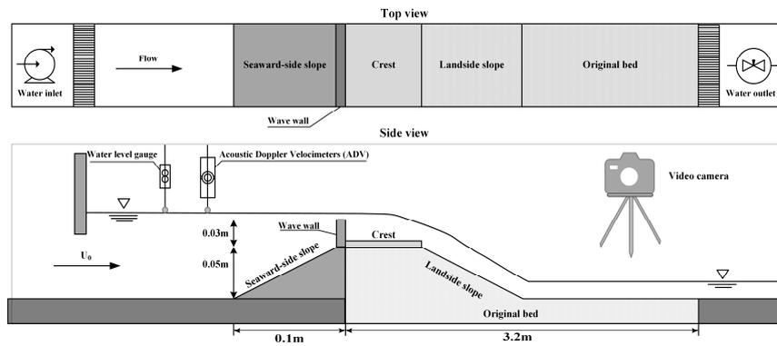
Fig 1. Schematic view of experimental setup.
