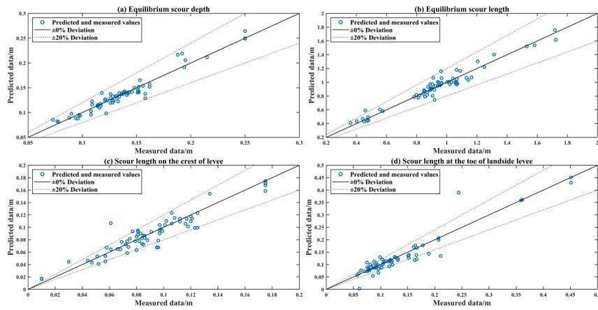
Fig 5. Comparison between predicted values with measured values in erosion features.
