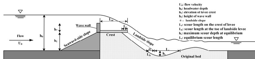
Fig 2. Schematic sketch of a scour hole around a levee during surge overflow.
